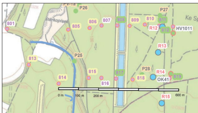
Fig. 4 Location of wells and data on levels of groundwater.
